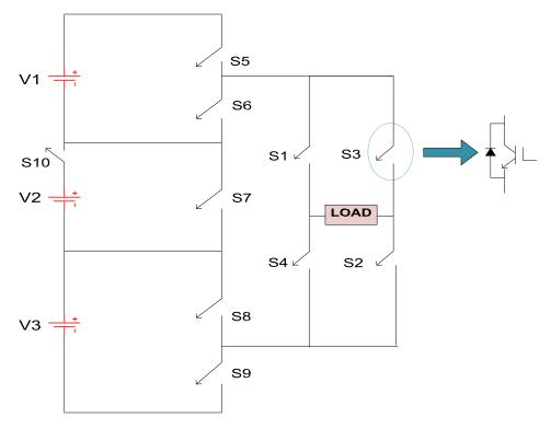
Explains the MLI operation during mode 6 and the output voltage in this mode is V2+V3=6V1. The maximum voltage occurs during mode 7 that is V1+V2+V3=7V1 and the MLI operation is explained. In the same way the negative cycle voltage can be obtained by following the switching operation explained in table 1. Power switches requirement with respect to output voltage level and comparison with the conventional asymmetrical CHBMLI and reduced H-bridge MLI [12].
